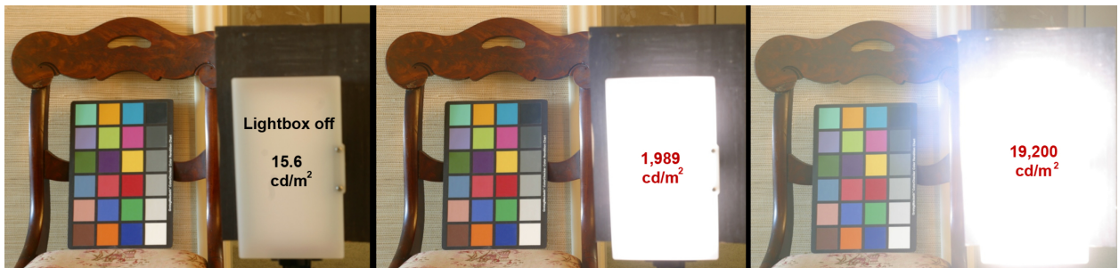
Figure 8.1 illustrates three of the five photographs using jpeg images. 8.1(left) shows the light box off; (right) shows maximum luminance. The lowest scene luminance was??
