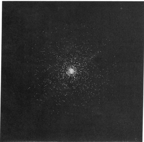
FIG. 3. Pattern of sensitivity for photometer reading of denominator. The angle from the center to the outermost dots (2.7 cm in this figure) is 12^\circ . One-half the dots are inside a circle of radius 2^\circ . (The corresponding radius of the numerator is 2 arc-min.) The density of dots, which was chosen empirically, here varies approximately as the inverse square of the radius.
