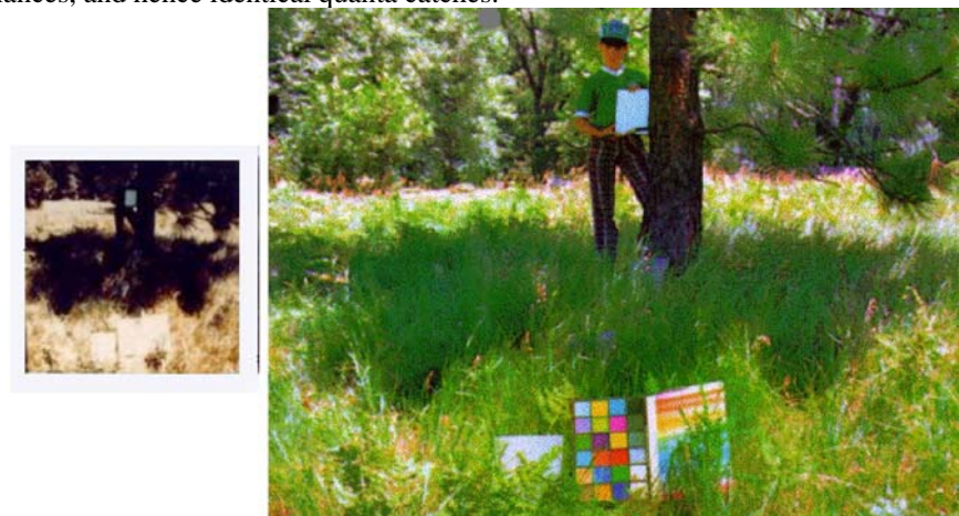
Figure 2 shows a pair of images of a boy holding a white card in the shade. The illumination in the sunlight was 30 times higher than in the shadow. Spot photometer measurements showed that the luminance of the black square in the test target was equal to the white card in the shade. The image on the left shows an S-shaped tone scale photograph taken at the time. All the detail in the sunlight has been lost. The right shows the results of spatial image processing from a digitized image scanned from a long-dynamic-range negative.
