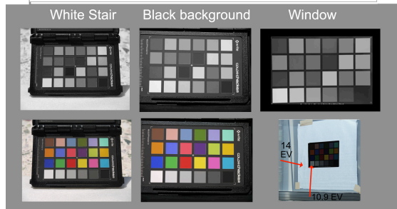
Figure 9 (top) Ratio of camera-estimated/actual reflectance vs. % max luminance in the field of view; (middle) The field of view (FOV) images of G separation captured by the camera; (bottom) the scenes: daylight on white stairs, darkroom on black, Window from Figure 8.
