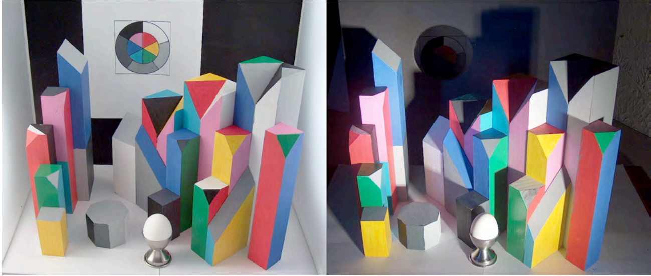
Figure 2. The pair 3-D Mondrians, made with 11 paints, viewed at the same time in the same room. The left is in nearly uniform illumination, while the right is in directional HDR illumination. Appearances vary with illumination, despite constant reflectances.
