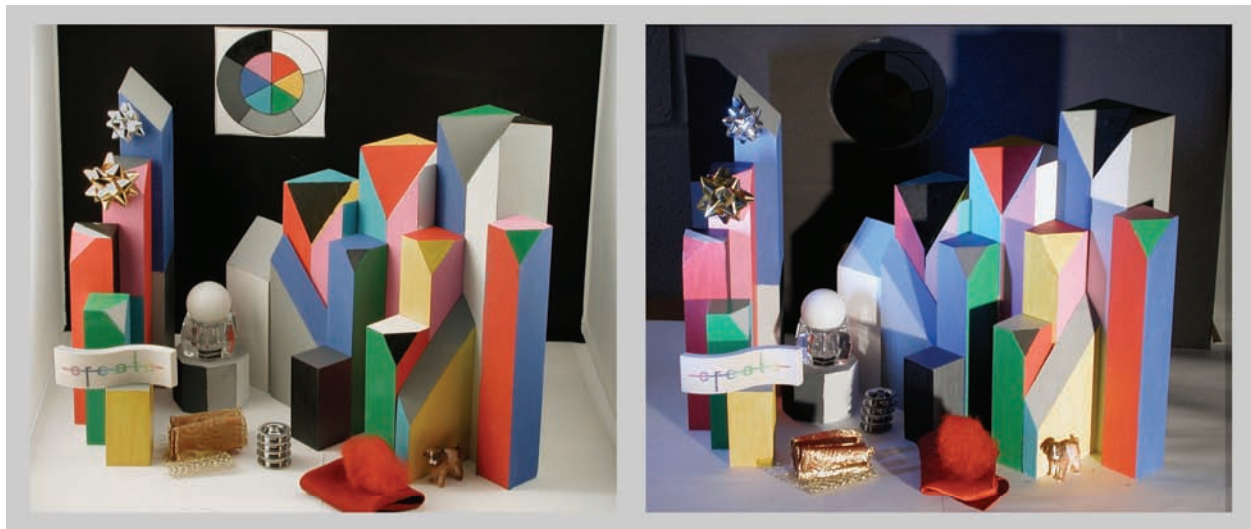
Figure 1a) shows the low-dynamic-range (LDR) scene on the left, and 1b) a high-dynamic-range (HDR) scene (right).
