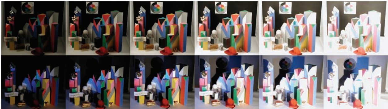
Figure 10 shows digital photographs of the low-dynamic-range (LDR) scene on the top, and photographs of the high-dynamic-range (HDR) scene on the bottom. Each photograph had twice the exposure of the one on its left. The photo on the far right had 64 times more exposure than the one on the far left. The exposure varied from 1/30 to 1 second.
