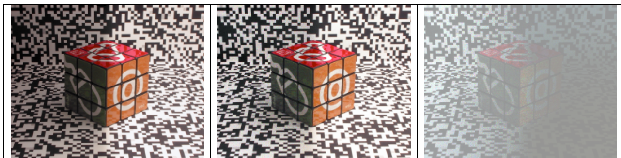
Fig. 6 – Object with shadow. Left the original, center the SCA filtered, right the difference image between the two [29].
