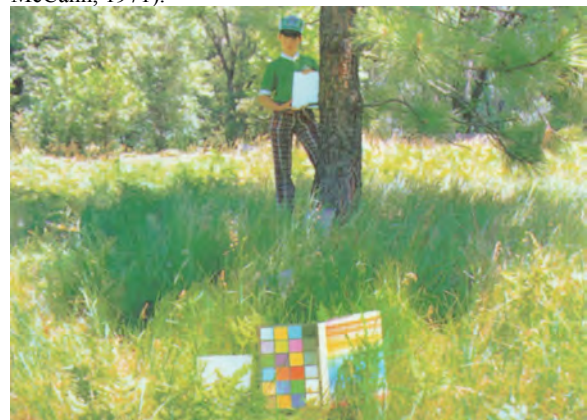
Figure 11 shows an example of an HDR scene processed with spatial comparisons (1978 Frankle and McCann patent application). The illumination on the white card in the shadow is 1/32 th that on the black square in the sun. Both the white card in shade and black square in sun have the same luminance. The spatial processing converted equal input digits ( -\log luminance) into very different output digits, thus rendering the HDR scene into the small range of the reflective print shown here.
